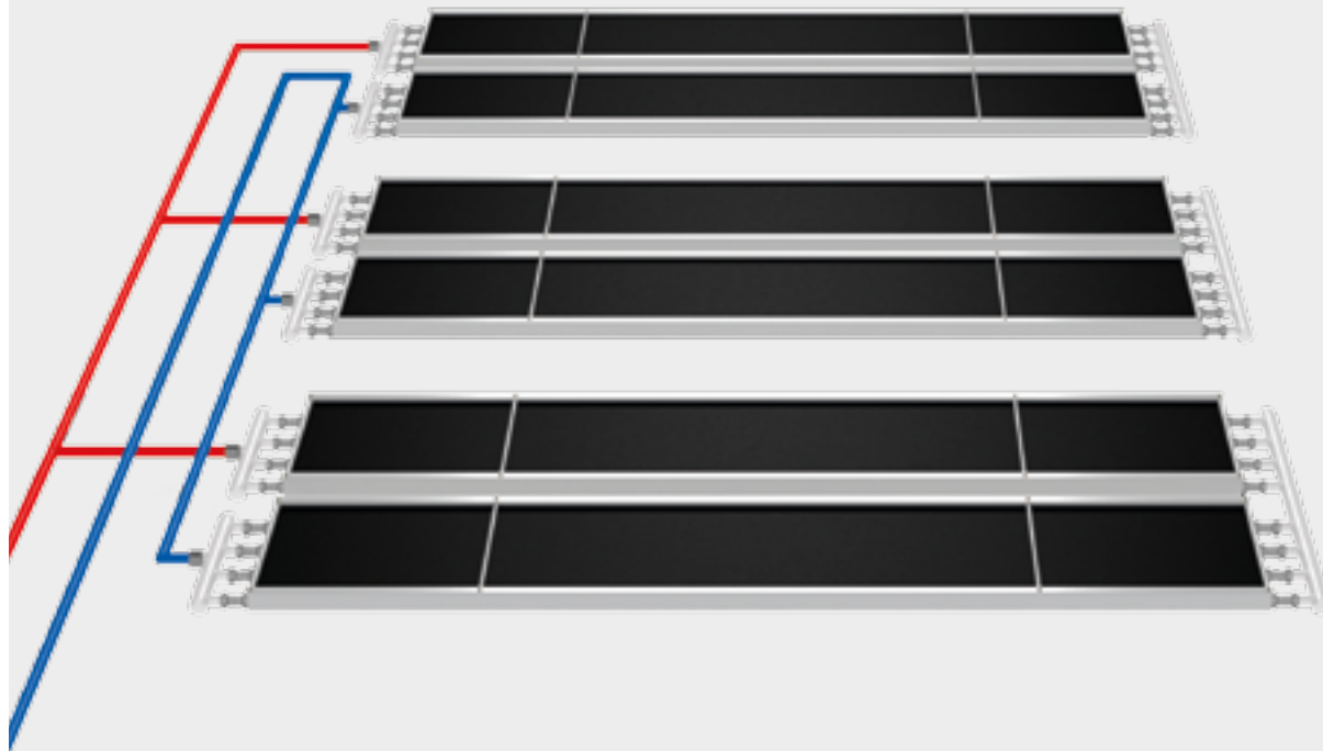
Fig. 1: Pipes laid according to the Tichelmann system (two-pipe system with reverse return)
